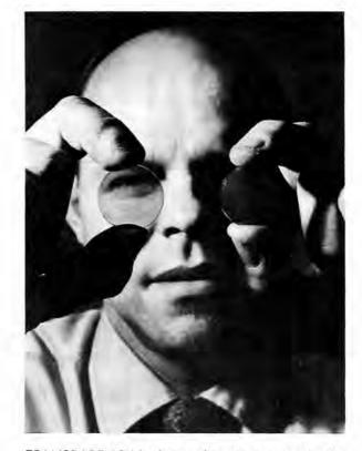
TRANSPARENCY is the goal in these ceramics for electro-optic applications, and Gene Haertling (2317) displays, at left, the improved transparency resulting from his new fabrication technique.
